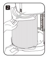
2. Remove the used filter and replace it with a new filter.
