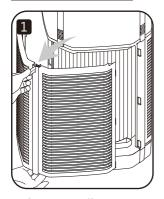
After turning off the power and unplugging the power plug, pull the filter cover tab behind the product backward.
